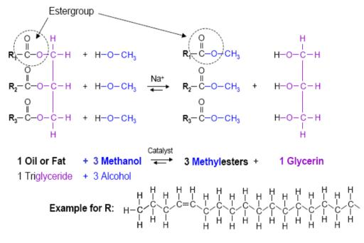
Figure1: Basic Scheme for Bio diesel production
